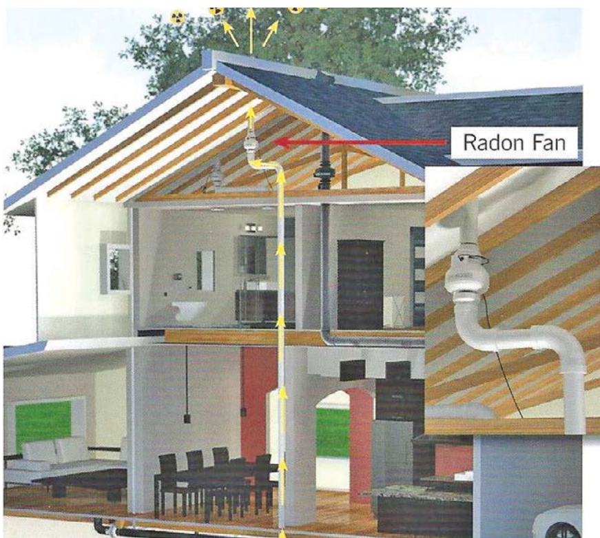
Newer homes may have built-in radon pipes, to which exhaust fans can be attached. (IMAGE WWW.MBRADON.COM/SERVICES)
