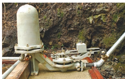
Welcome to the water hammer. This device by Rife, which has been around since before the Civil War, is called a RAM pump. There are many YouTube videos of this pump doing its magic. Check it out.
